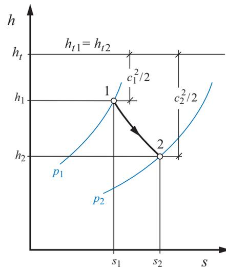
g) Exergiebilanz:  $0 = e_1 - e_2 + \frac{1}{2}(c_1^2 - c_2^2) - e_V, \quad e_1 - e_2 = h_1 - h_2 - T_u(s_1 - s_2)$
