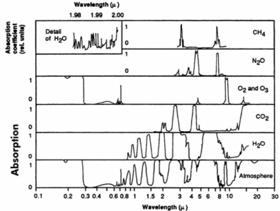
Figure 5-2. Absorption spectra for  $\text{CH}_4$ ,  $\text{NO}_2$ ,  $\text{O}_2$ ,  $\text{O}_3$ ,  $\text{CO}_2$ , and  $\text{H}_2\text{O}$ , and of the atmosphere. (From R. G. Fleagle and J. A. Businger [2006] after J. H. Howard [519] and R. M. Goody and G. D. Robinson [514])
